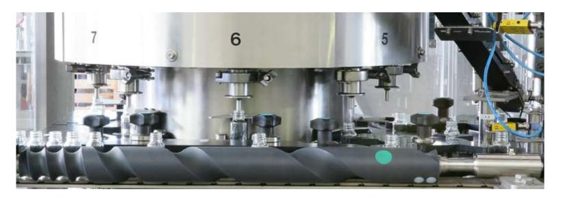
The **FF Series** of Monobloc rotary filling and capping machines is the result of over 15 years of activity in the field of liquid filling. The FF Series is supplied in two versions. The FF-P series is for Pharmaceutical applications and the FF-G Series is for Cosmetic, Personal care, House-Hold Care and Food applications. The FF Series is modular, flexible and offers the Pharmaceutical, Cosmetic, Personal care, House-Hold Care and Food industries the right technological filling solutions.
