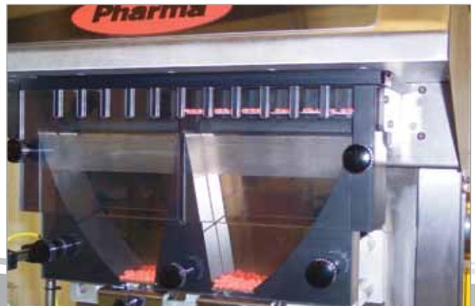
don't require any routine calibration. This factor therefore removes the maintenance costs associated with such an operation. The count heads are virtually immune to dust and will count all products with high accuracy from 2.5mm in size.
