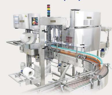
Autopack SLO Bundle Shrink Wrapper with welding bar is the ideal solution for collation and wrapping of oval shaped containers. Depending on speed and shape, the machine can be configured with or without feed screw. It is among the most compact solutions on the market, available in single, double even triple track configuration for speed up to 50 packs/min.
