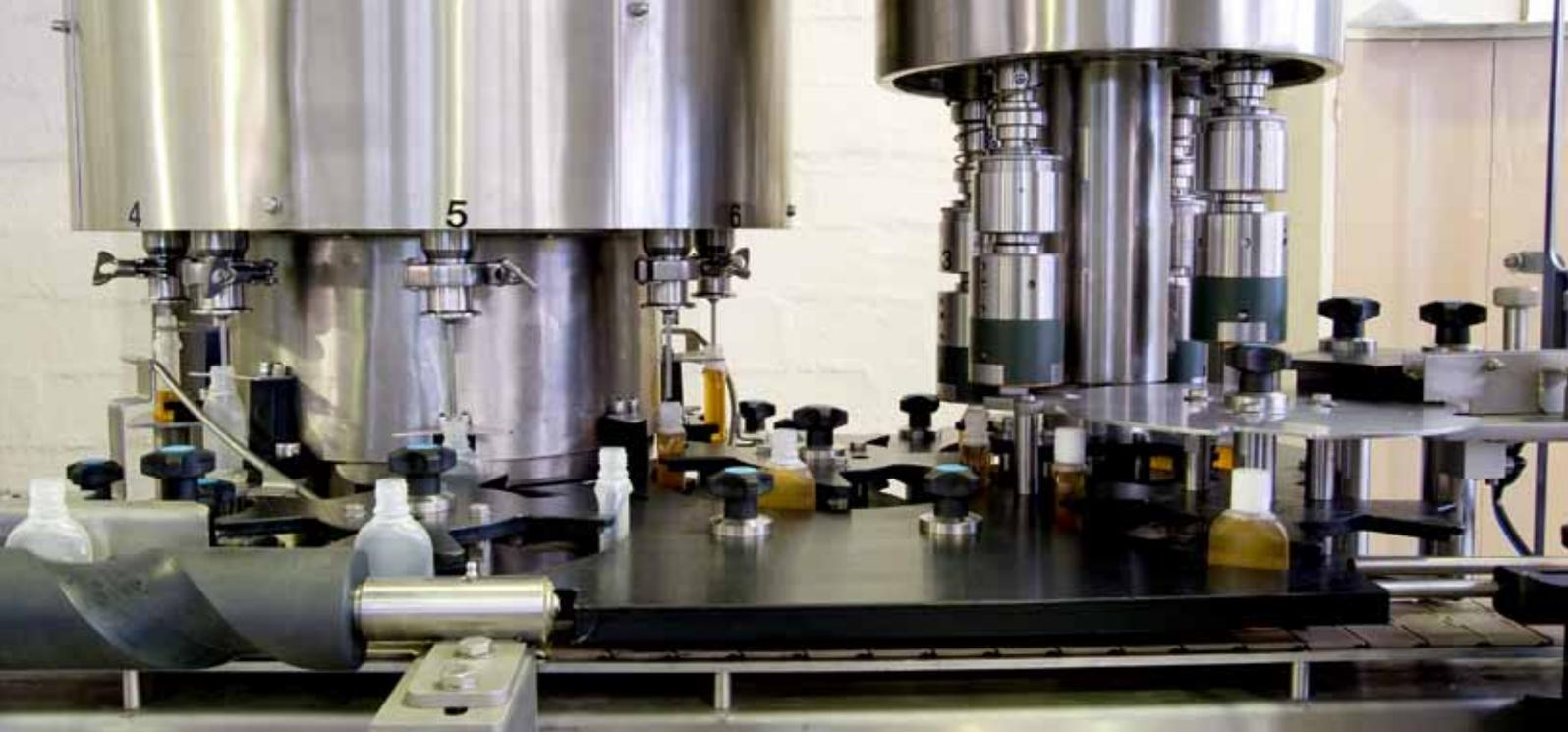
Level Filler option: Level filling turrets are used for low viscosity liquids only. The containers are lifted on a cam, thus opening the level nozzles with filling automatically stopping at the required fill height. The fill height is simply adjusted by adding or removing spacer rings from the nozzles.
