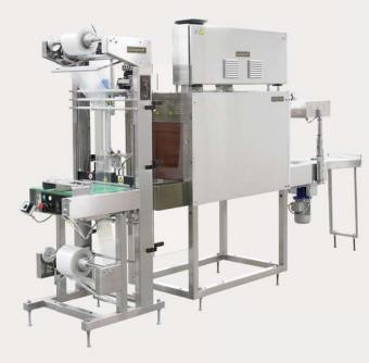
Autopack SSO is a Semi-Automatic Bundle Shrink Wrapper particularly suited for low speed application and/or contract packaging when product size, collation change many times per day. Product collation and pushing through the film is by operator, pneumatic pusher optional. Welding bar descends automatically only when the pusher is drawn back to home position to ensure operator safety.
