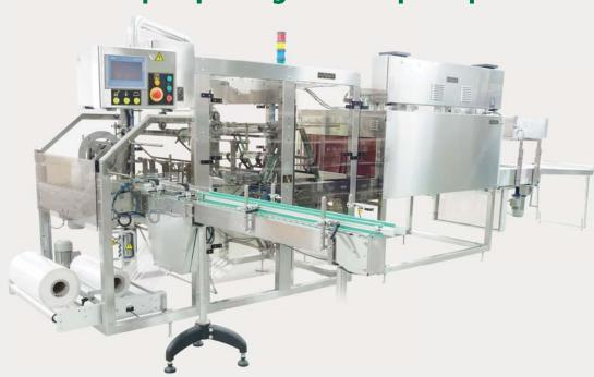
Autopack SLA / SLR CMOS is a Continuous Motion Overlap Seal bundle shrink wrapper with Side infeed for Aseptic packages and square products. With a maximum speed of 45 cycles/min, it is Autopack's fastest machine and among the world's most compact overlap seal machines with speed of up to 135 packs/min (triple tracks).
