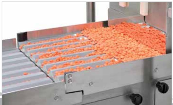
Conveyor and reject system controls are configurable from within the control system to allow total process control and full statistical data is stored and can be printed if required.
